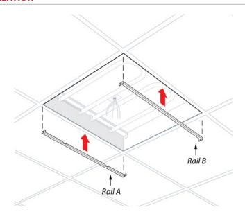
The mounting rails are inserted between the troffer and grid rail on oppositie sides with the anti-rotational tabs pointed inward and notches facing up.
